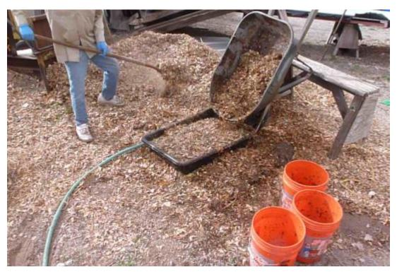
Figure 6. Setup for Wetting Feed Materials
